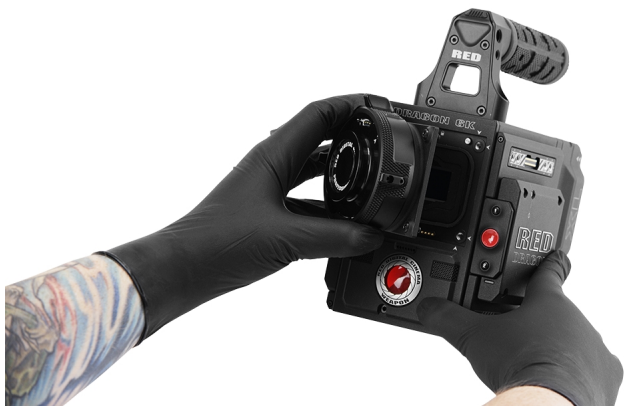
Figure: Align Lens Mount Pins
