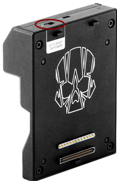
Figure: Auto Boot on Power Switch
