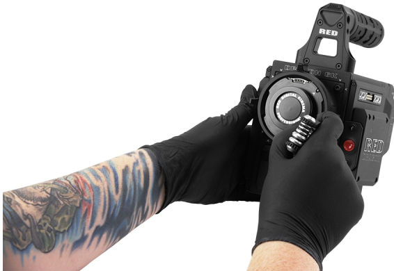
Figure: Remove the Lens Mount Screws
