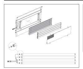
The FreeStyle T44/T24 fixture is comprised of a Louver, Reflector and Tube Harness.
